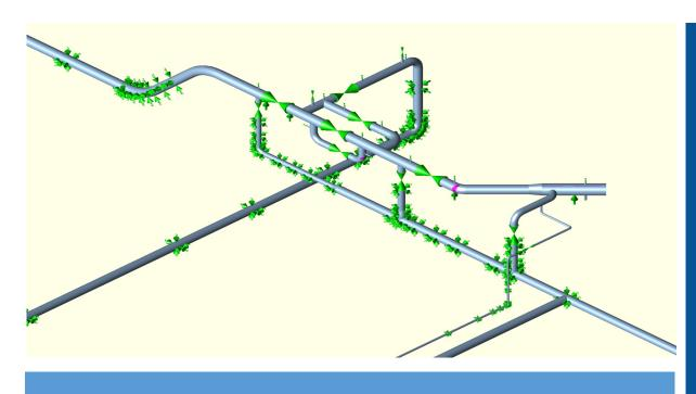
SPEC performs detailed engineering evaluations of existing and proposed piping systems for structural adequacy and in support of expansion loop and pipe support design using industry standards and commercial software. This includes static and dynamic analyses as well as evaluation of surface loads on buried pipelines. Depending on the scope of the project, SPEC deliverables can range from stand-alone design reports to complete design and fabrication packages.
